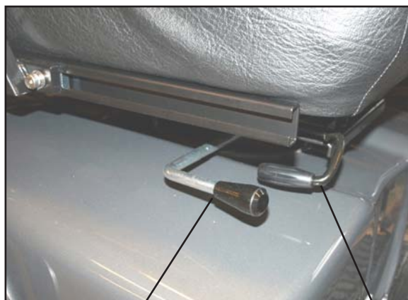
Release lever for seat rotation. Release lever for seat forward/back.
